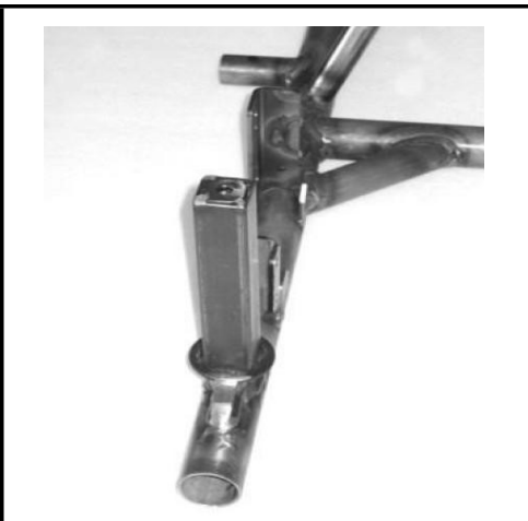
Photo of the frame from the back with the section of the support for the RTPS (Rear Tire Protection System).
