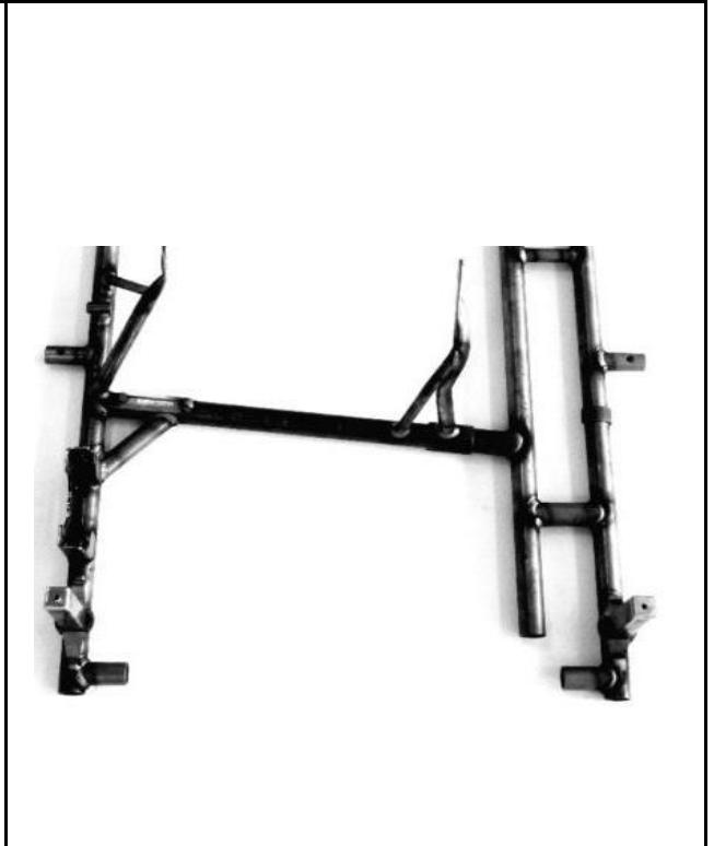
Photo from above of the frame with the section of the two supports for the RTPS (Rear Tire Protection System)
